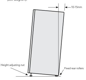
3. Wind the large height adjusting nut on the handle side down until the refrigerator is level and stable. If you have difficulty winding the nut or height adjusting foot down, have someone tilt the refrigerator back so you have better
